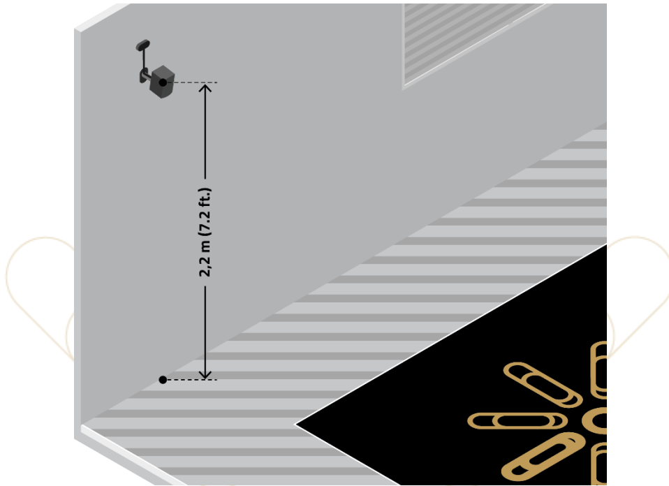
Figure 4 - Base station distance above the ground
