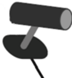
Figure 11 - Mount the sensor on the holder
