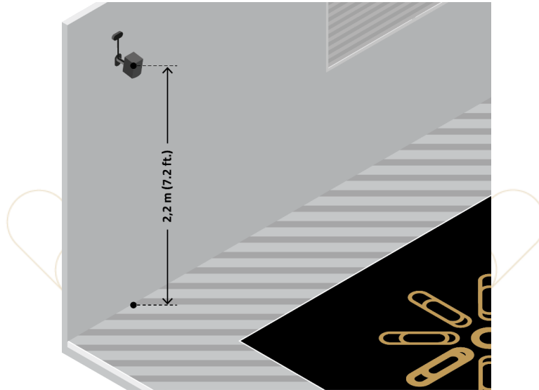
Figure 4 - Base station distance above the ground
