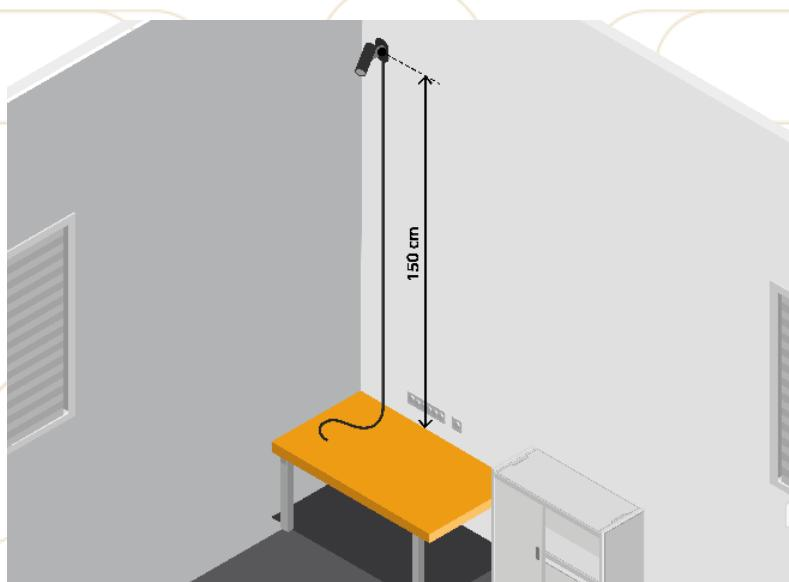
Figure 7 - HTC wireless link box mount option 2
