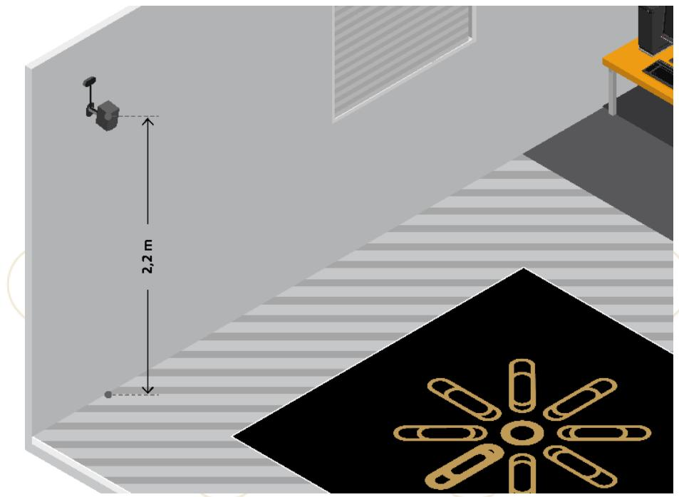
Figure 4 - Base station distance above the ground
